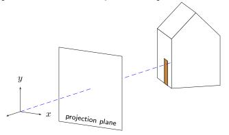
The way we constructed the points of the house now makes it easy to draw rays of projection. We'll cast one ray from every visible vertex of the house and define options so the appearance of all rays can be changed at the same time.
